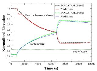
Fig. 3 Comparison of normalized experimental RPV and containment collapsed liquid level with NRELAP code predictions for blowdown event.
