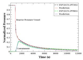
Fig. 2 Comparison of normalized experimental RPV and containment pressure with NRELAP code predictions for blowdown event.
