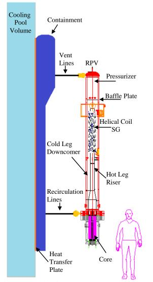
Fig. 1 Schematic of the NuScale Integral System Test (NIST) facility and major components.
